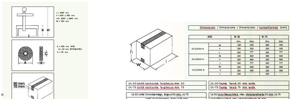
Diagram illustrating the dimensions of the SC1/500-A tape sealer:
